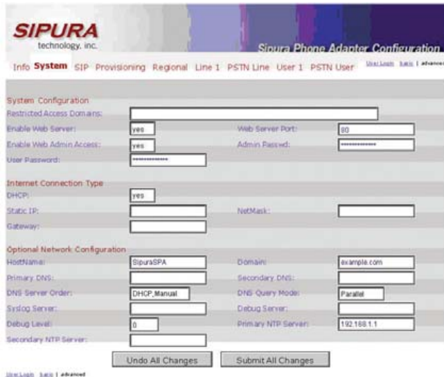
Figure 2. Use the Web interface to set up the Sipura 3000.
