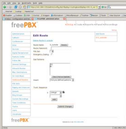
Figure 17. Handling 9 for Outside Lines and 911 Separately
