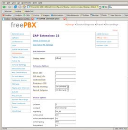
Figure 10. Default device options are sufficient for ZAP extension 22.
