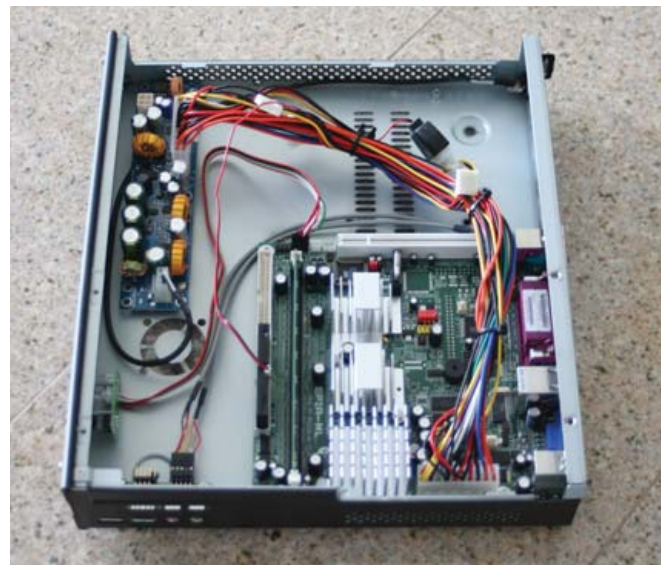
Figure 2. The Open Casetronic Case with Motherboard
