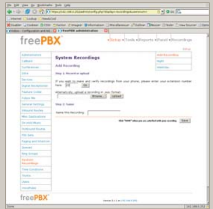
Figure 18. Set up an outgoing recording from extension 22.
