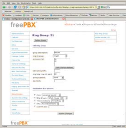
Figure 16. Ringing the Whole House from an Extension
