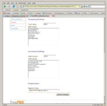
Figure 9. Configuration of the IAX2 Trunk
