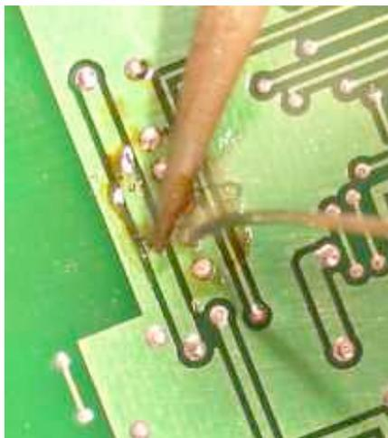
6. Solder the remaining down, and inspect the joints. The underneath pad is almost impossible to inspect unless you have some sort of access to X-Ray equipment unfortunately.
