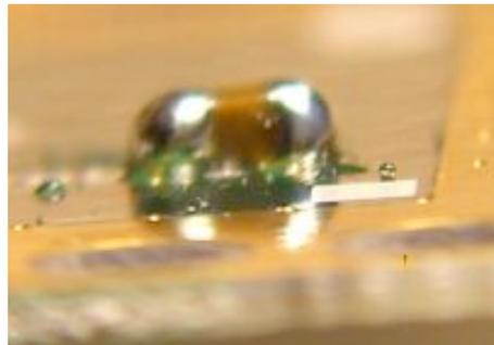
Remember that you should have the soldering iron on the device for under two seconds. If something isn't working out (for example you lose grip of the device and it swivels as the solder melts), it might be best to simply remove your
