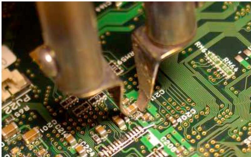
This method is fast and easy, and probably the best. The downside is you have to have the **hot tweezers** (some soldering stations offer these as an attachment as well). The house powered version heats up very fast, but it also stays at a fairly high temperature. This means you must be fast or you will burn the part.
