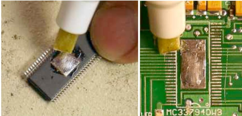
4. Position IC in proper place, and solder one of the pins on the IC down to hold it in place.
