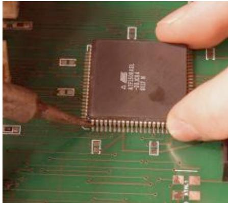
4. Inspect the entire device and see how the pins line up. If all went well in step 3 all of the pins will line up. If they don't, remelt the one pin that is soldered and use tweezers to nudge the device into alignment. Be careful though, with only the one pin soldered in if you bump the board you might shift the part and bend the pin.
