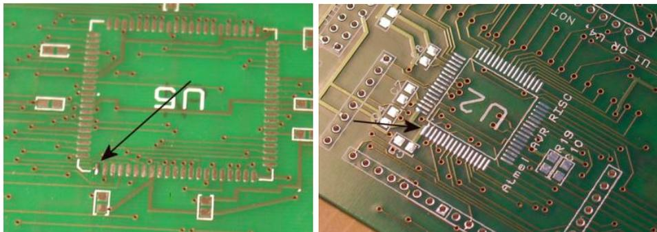
2. Apply flux over all the pads of the IC that will be soldered. One pass should be enough flux, you don't need or want a massive amount of flux on the board. However you may need additional passes, as most of the time two little flux will probably be a bigger problem than too much. Try one or two passes at first, and you should get a feel for the flux pen and how the flux effects the soldering process.
