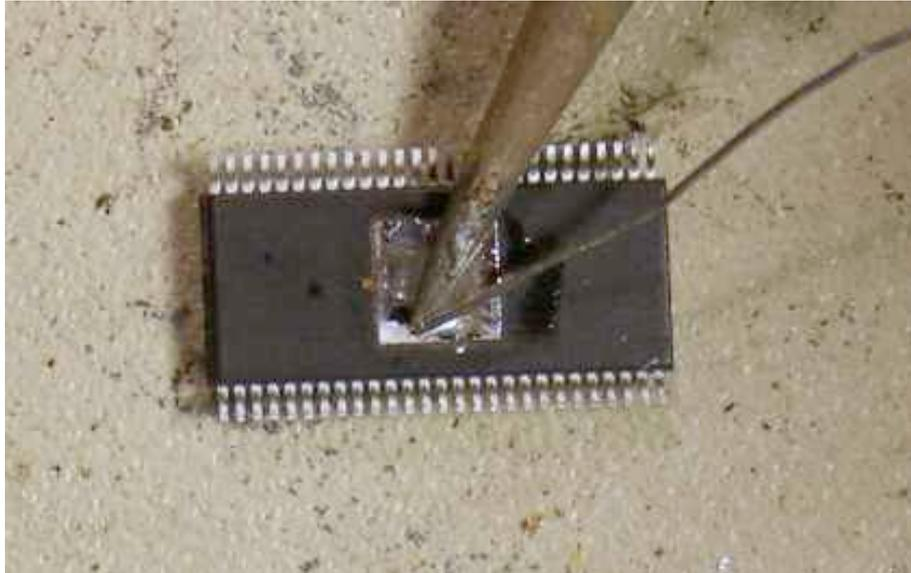
2. Add a tiny bit of solder to the pad on the PCB, again later most of the solder shown in the picture was removed with solder wick.
