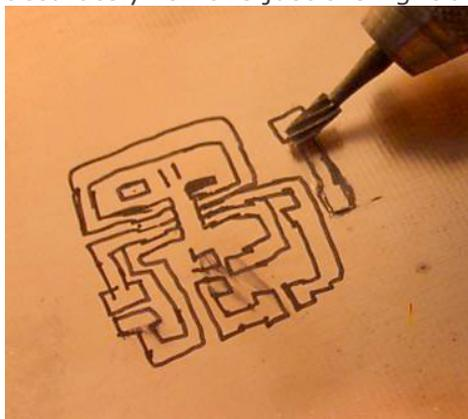
4. Check for shorts or spots you didn't remove the copper on (use inspection visually and with a continuity check)
